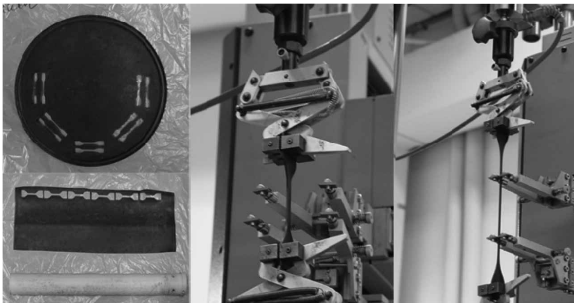
Figure 1 | Material sampling method from disc (left top) and tube diffusers (left bottom) and implementation of the stress strain tests (middle and right).
