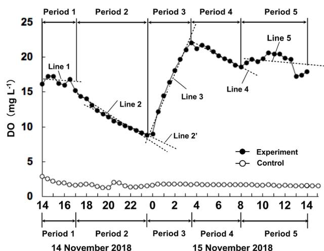
**Figure 3:** A typical example of the diurnal DO fluctuations monitored every thirty minutes between 14:00 on 14 November and 15:00 on 15 November 2018. They were divided into five different periods (Period 1 to Period 5), and a regression line was interpolated to the data plots in each of the five periods.
